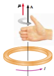
Figure 29.15 Right-hand rule for determining the direction of the vector \mathbf{A} . The direction of the magnetic moment \boldsymbol{\mu} is the same as the direction of \mathbf{A} .
