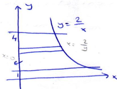
$$V = \pi \int_1^4 \left( \frac{2}{y} \right)^2 dy = 4\pi \left[ -\frac{1}{y} \right]_1^4 = \frac{3\pi}{4}$$
